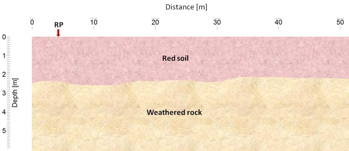
Figure 4. Litholog of the trench excavated at line 2 (IISc Campus site) showing a red soil layer and a lower weathered rock layer.
