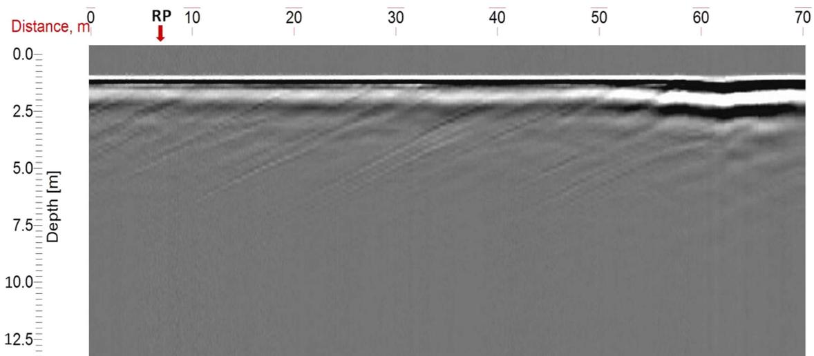
Figure 7. Typical GPR profile of raw data collected by using the 25 MHz antenna from line 1 (IISc Campus site).
