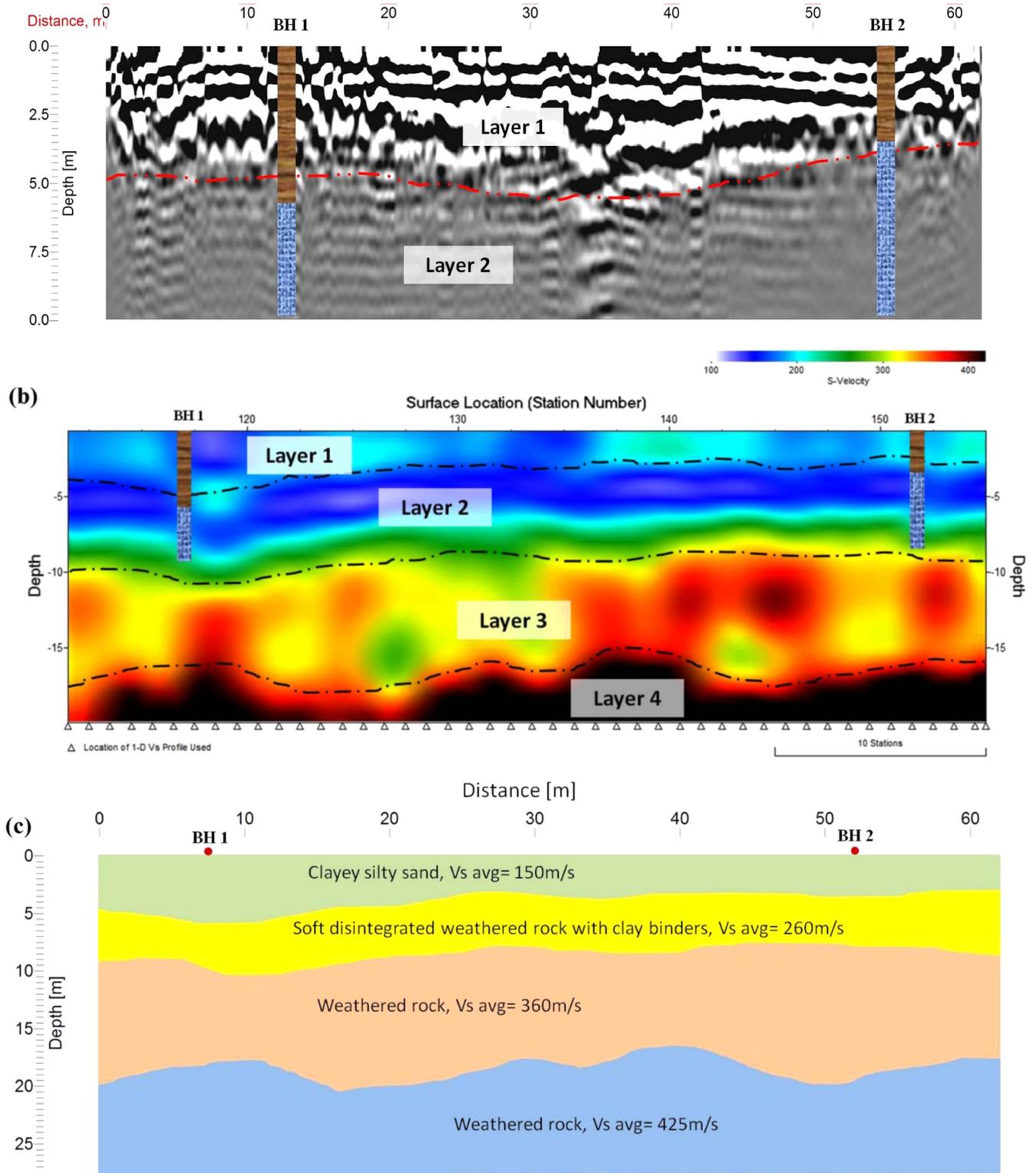
**Figure 13.** (a) GPR profile of line 3 after all corrections at the Whitefield site. (b) 2D MASW profile of line 3 at Whitefield site. (c) Final subsurface profile of line 3 at the Whitefield site by comparing all the methods.
