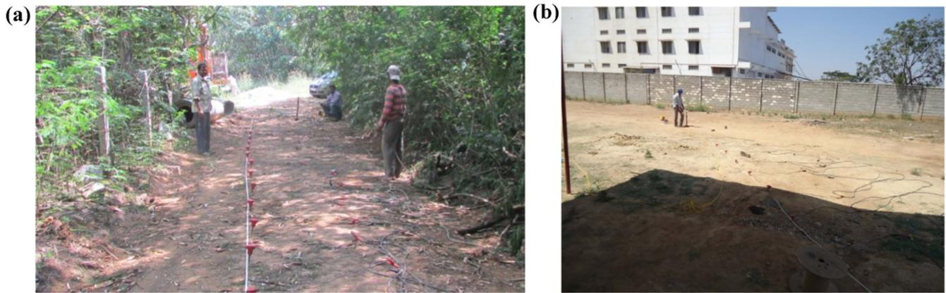
**Figure 8.** MASW data acquisition in the field using 4.5 Hz geophones and a 24-channel geode (a) at the IISc site and (b) at the Whitefield site.
