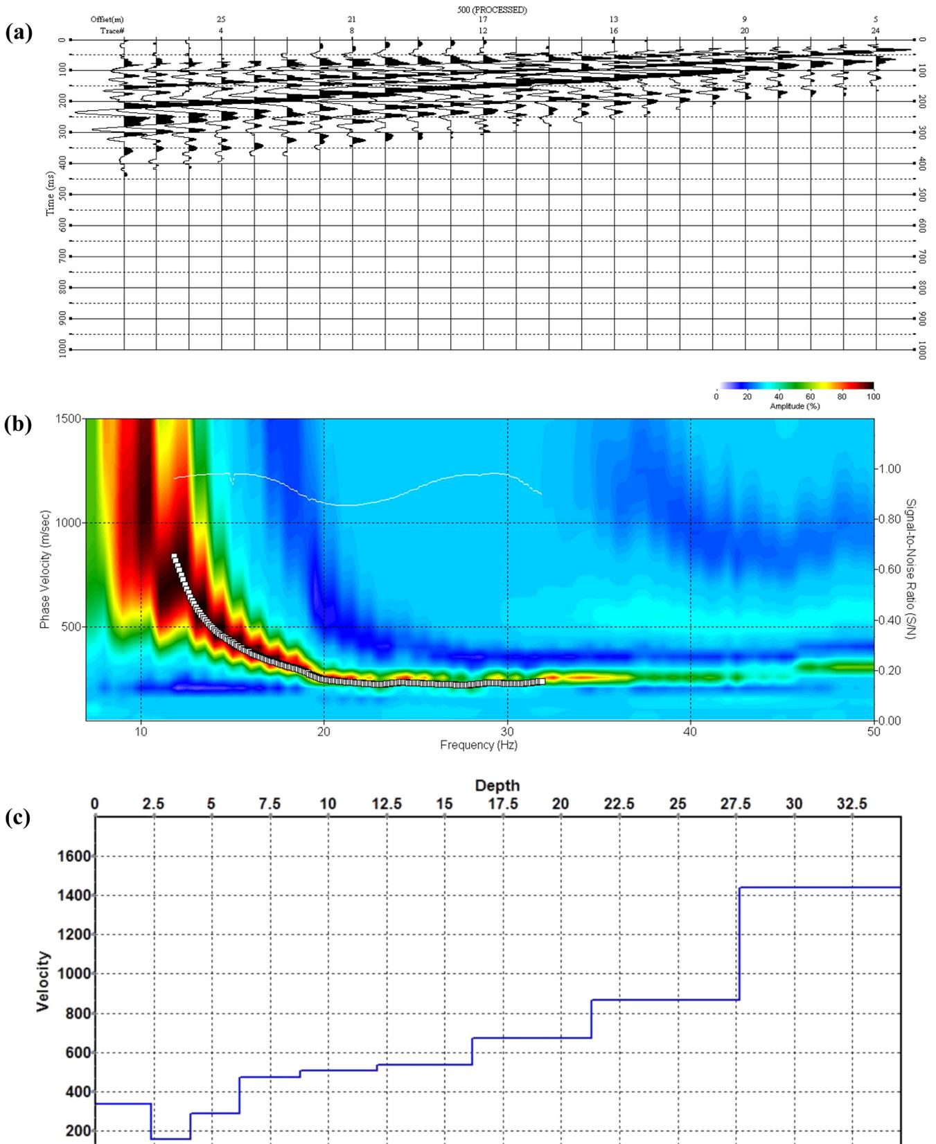
**Figure 9.** (a) Time domain raw seismic data with multi-shot surface wave roll. (b) Extracted dispersion curve. (c) Typical inverted 1D velocity depth profile for the IISc Campus site.
