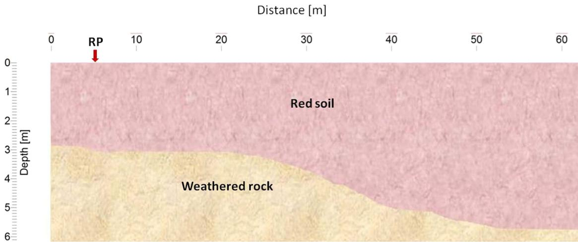
Figure 3. Litholog of the trench excavated at line 1 (IISc Campus site) showing a top layer of red soil and a lower layer of weathered rock.
