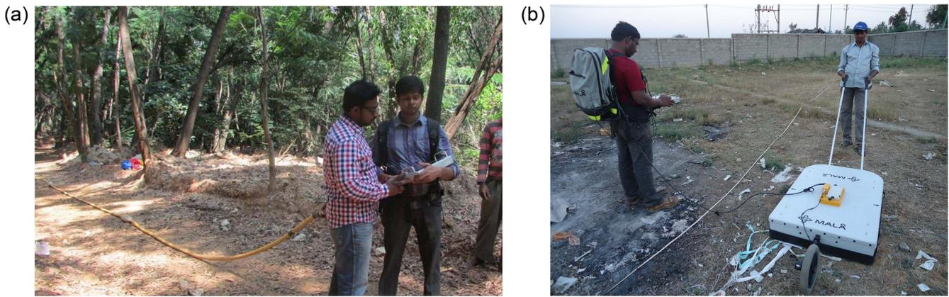
Figure 6. GPR data acquisition in the field. (a) 25 MHz antenna at the IISc campus site, (b) 100 MHz antenna at the Whitefield site.
