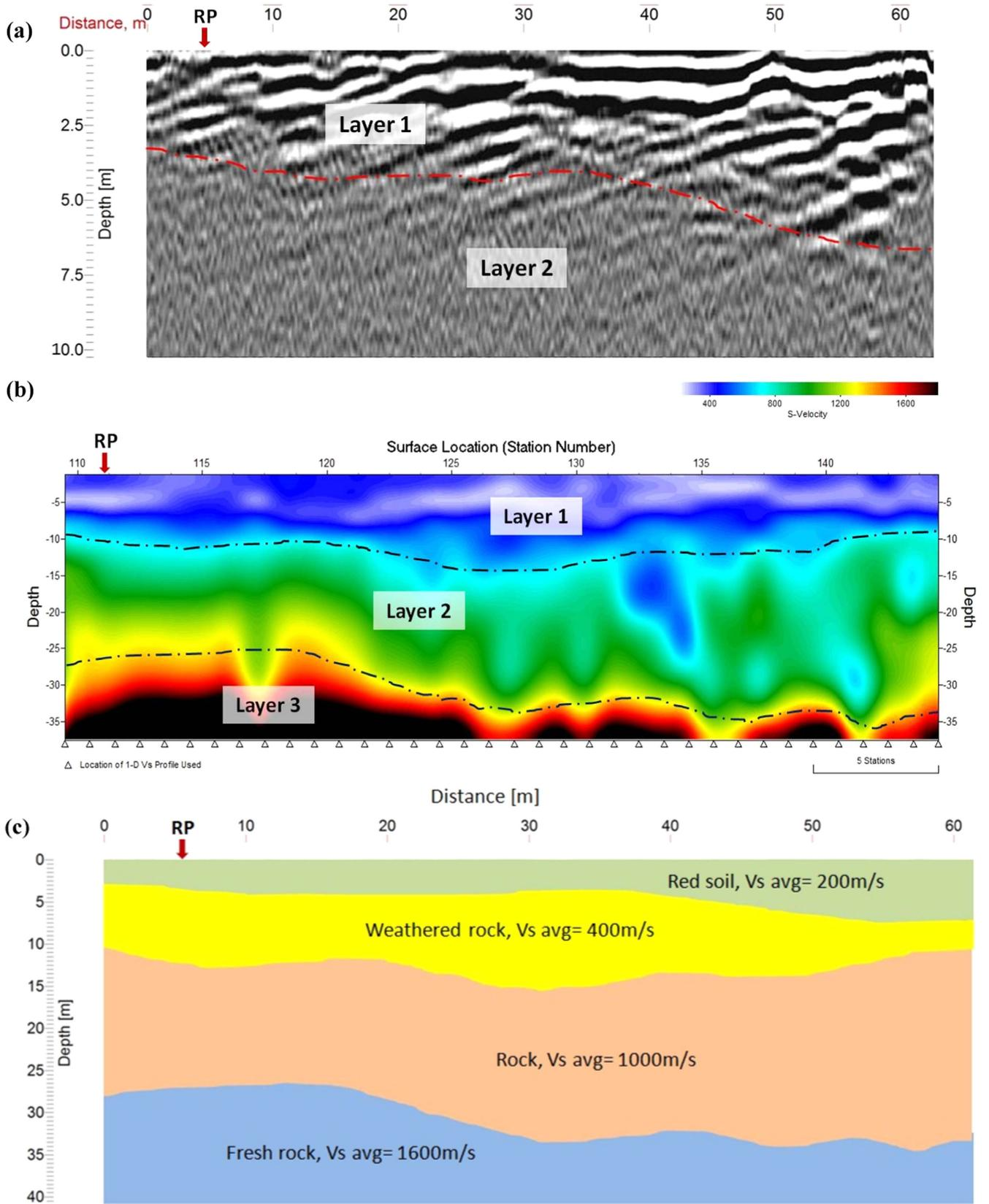
**Figure 11.** (a) GPR profile of line 1 after all corrections at the IISc Campus site. (b) 2D MASW profile of line 1 at the IISc Campus site. (c) Final subsurface profile of line 1 at the IISc Campus site by comparing all the methods.
