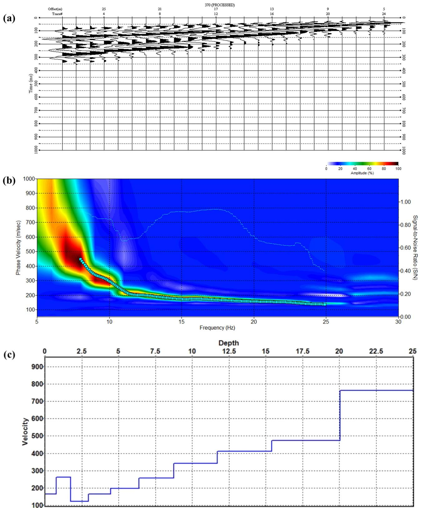
**Figure 10.** (a) Time domain raw seismic data with multi-shot surface wave roll. (b) Extracted dispersion curve. (c) Typical inverted 1D velocity depth profile for the Whitefield site.
